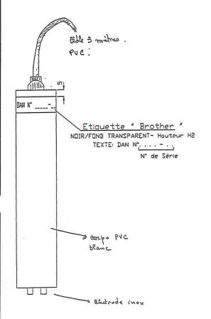
532050 - DAN-DETECTEUR DE NIVEAU ENSEMBLE RELAIS/BUZZER/ELECTRODE 220V/50HZ
