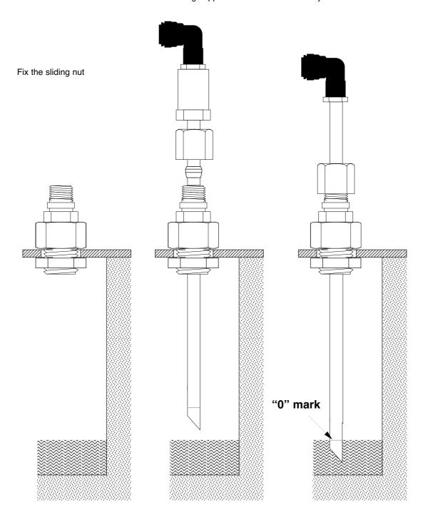
The height of level "0 flow rate" is always the same, repositioning after cleaning is then easy.
