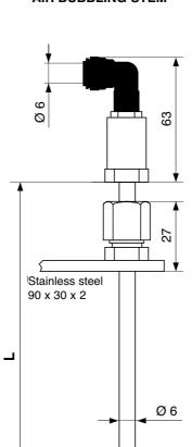
The BAMOBUL must be connected to the air bubbling stem immersed in the liquid.
