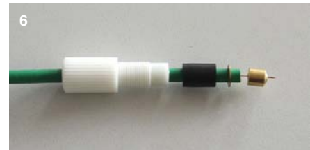
6 placing brass turning piece (ca. \varnothing 8 \times 8.5\text{mm} , tip with cone)
