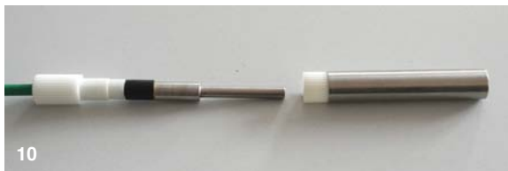
10 Putting on the coaxial cable and screwing it with the upper part
