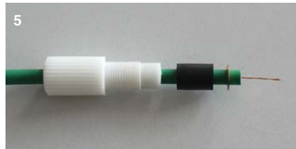
5 Placing brass washer ( \varnothing 10 \times 2 - 0.6\text{mm} )
