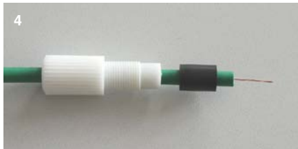
4 Placing neoprene sealing ( \varnothing 10.5 \times 2 - 14.5\text{mm} )
