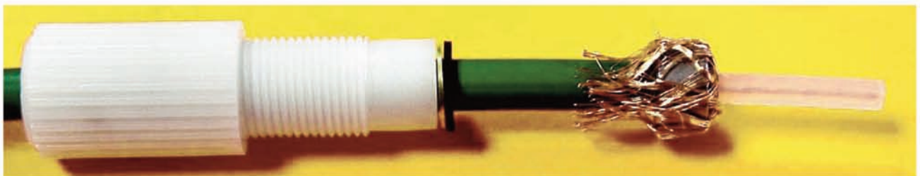
Sliding the stainless steel ring to the leading edge of the coating and putting the shield over it.
