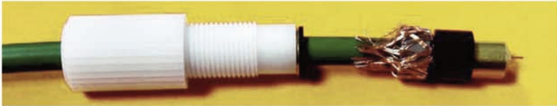
Beading on of the neoprene pressing piece and brass turning piece
