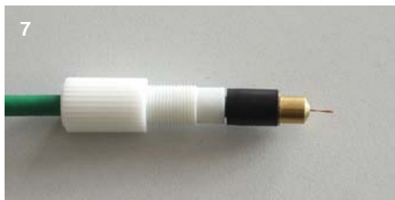
7 Placing brass turning piece up till cable coating
