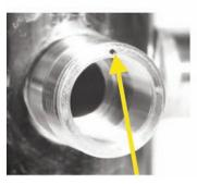
Observe the positioning of hole and pin.
