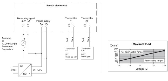
**NOTE:** The measuring output "4-20 mA" is a current drain, this means, the output channel has the same electrical behaviour as a variable resistor. An active power supply for the measuring circuit is always needed.
