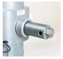
1) Screw the ETR-glass with the included tool and remove.
