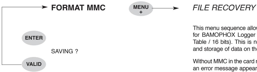
This menu sequence allows the format of Memory card for BAMOPHOX Logger as a FAT 16 (File Allocation Table / 16 bits). This is necessary to assure recording and storage of data on the Memory card.
