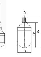
With the built-in ballast, it is no more necessary to fix a switching point along the cable.
